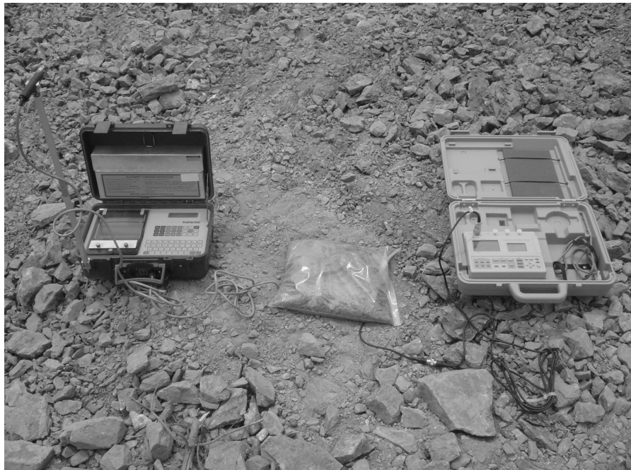
Fig. 2. A picture of installed Blastmate and Vm-53.
