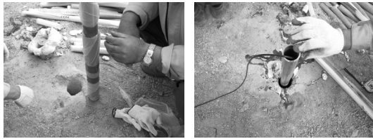
Fig. 5. The process of inserting Al-foot's sensor into the bore hole.
