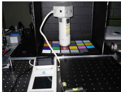
Fig. 2. RGB color detection system (Konica Minolta, CR-400, JAPAN).
