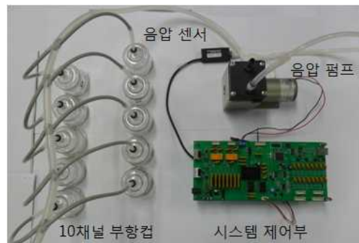
Fig. 1. Experiment setup for evaluation of skin pigmentation.
