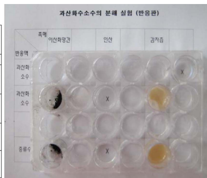
Fig. 7. SSC experimental apparatus developed for decomposition of 30% and 3% hydrogen peroxide.
