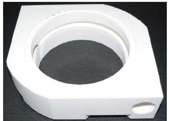
Fig. 5 Twin spiral case manufactured by rapid-prototyping machine.
