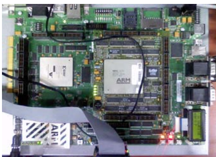
Fig. 8. Evaluation board with an ARM11 MPMC09 core tile
