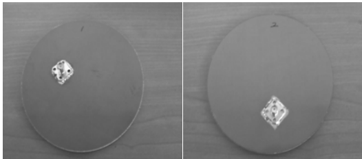
Fig. 5. 850MHz and 2.4GHz Antenna shape
