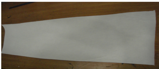
(c) Separator between anode and cathode
