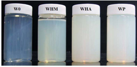
Fig. 3. Photographs of acrylic terminated polyurethanes prepared with different types of acrylate monomers in Table 1.
