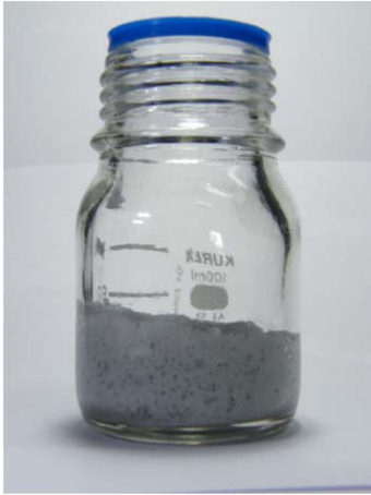
Fig. 3. Photograph of gel formed after NaBH 4 hydrolysis reaction.
