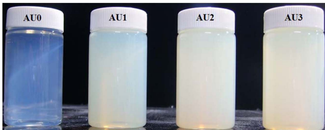
Fig. 4. Photographs of acrylic terminated prepolymers prepared with different moles of PETA in Table 1.
