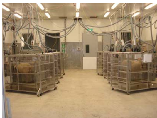
Plate 2. Measuring CH 4 from sheep emissions in purpose built CH 4 calorimeters.
