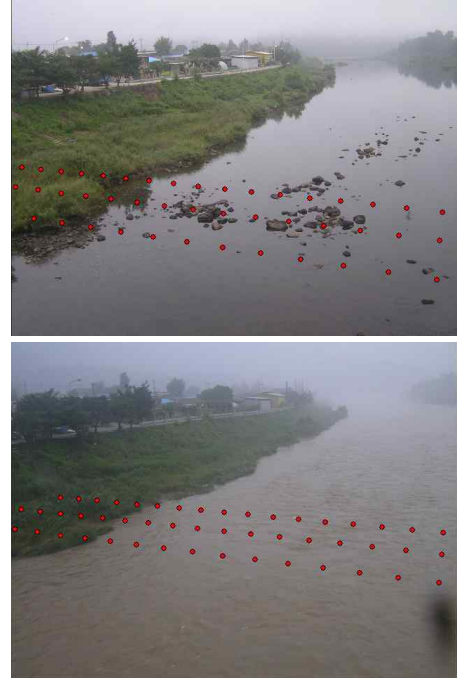
Fig. 4. Change of Measurement Lines Due to Water Stage Change. (upper right: low water stage, lower right: high water stage)
