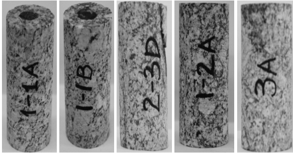
Fig. 3. Weathered rock core samples
