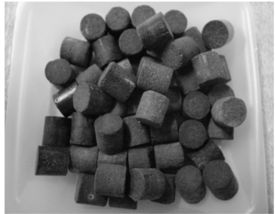
Fig. 1 Pellet type Cu-ZnO/Al 2 O 3 catalyst for WGS at high pressure condition
