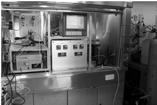
Fig. 4 PEMFC test station
