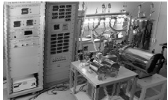
Fig. 16 Test rig for in-bed calorimetry
