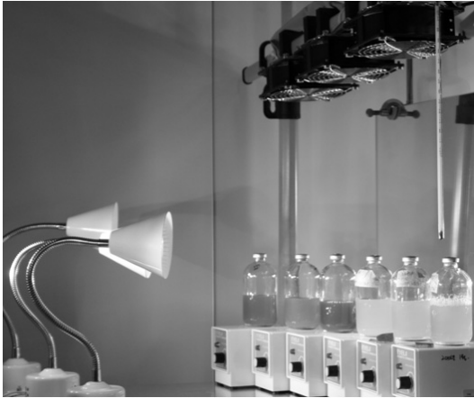
Fig. 1 Experimental setting for photo-fermentation
