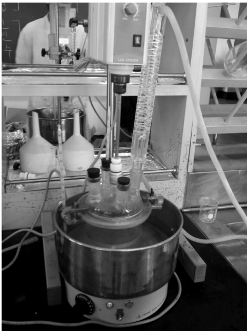
Figure 1. Experimental apparatus for multi core-shell polymerization.
