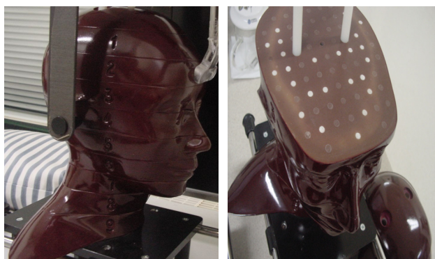
Fig. 1. Head & Neck phantom with 3×3 cm hole grid spacing and 5 mm hole diameter (levels 0-9)
