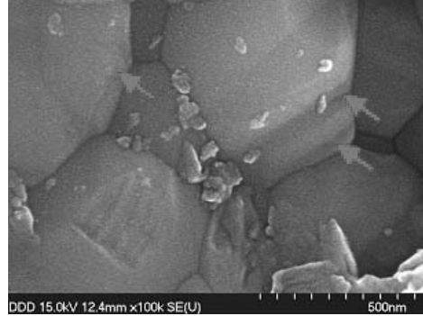
Fig. 6. Specimen DDD: surface grains of Y-TZP after etch removal porcelain applied with distilled water fired at 750°C.
