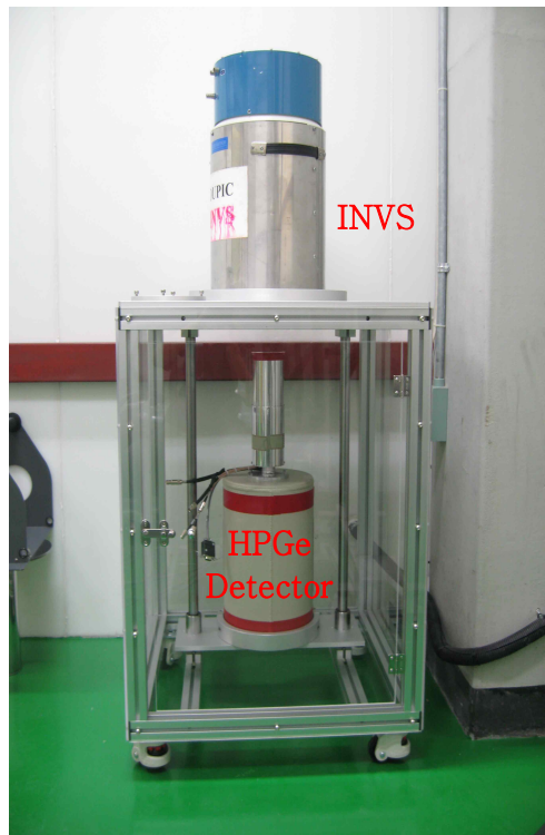
Fig. 1. Setup of gamma-ray detector.
