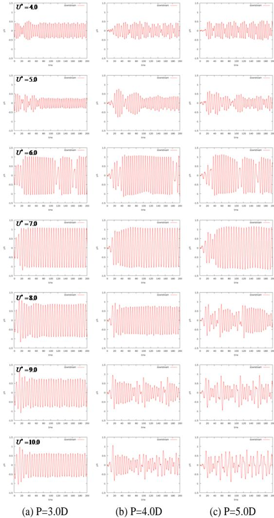
Fig. 17. Amplitude histories at downstream cylinder
