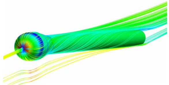
Fig. 7 . Stream line plot at M=0.85 and \alpha = 6^\circ
