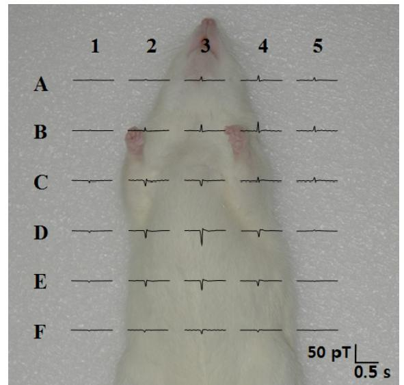
Fig. 4. MCG waveform distribution depending on measurement position.
