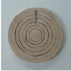
Fig. 2. The circumferential slices cut from log cross section to survey a distribution of the final moisture content in the radial direction of L-specimens.
