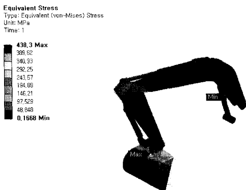
Fig. 11 Contour of equivalent stress at excavator
