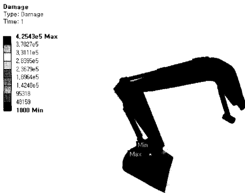
Fig. 16 Contour of damage at excavator
