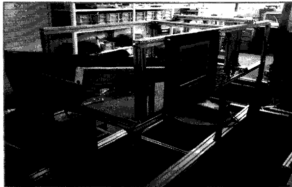
Fig. 6. Color sorting system for waste fireproof material.
