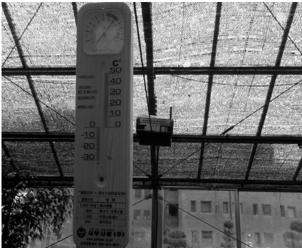
Fig. 5 Temperature calibration of an USN node with an analog thermometer.
