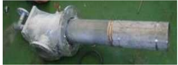
Fig. 5 125,000 kcal/h industrial RT burner equipped in the laboratory testing facility
