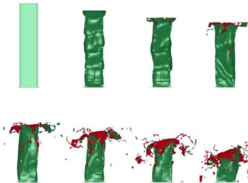
**Fig. 3** The collapse shape of 15° member in simulation
