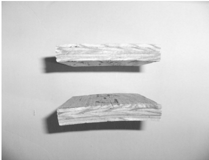
Fig. 2. Cupping of tested LVL after soaking and drying cycle treatment under the test standard.
