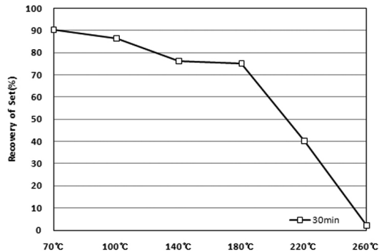
Fig. 5. Relationships between recovery of set and compression temperature of heat-compressed wood.
