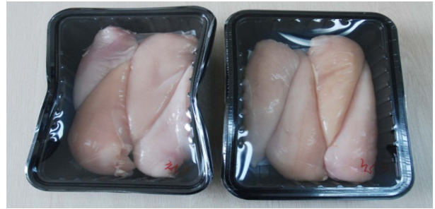
Fig. 1. Tray collapse of packed chicken with modified atmosphere with CO 2 and N 2 . Left: Packed chicken with an atmosphere containing 60% CO 2 and 40% N 2 , Right: Packed chicken with an atmosphere containing 40% CO 2 and 60% N 2 .
