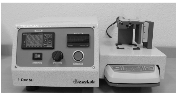
Fig. 2. Apparatus for grindability test
