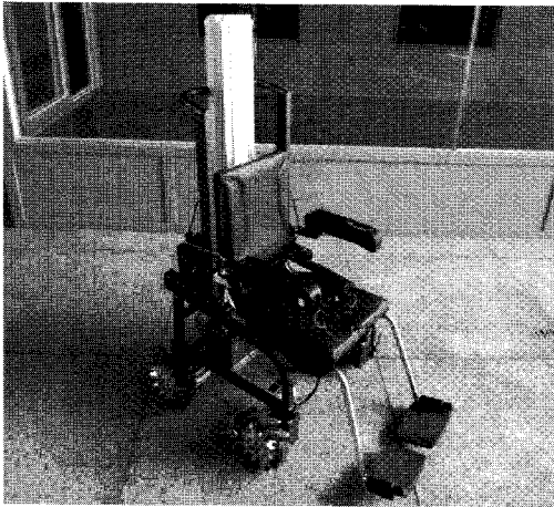
Fig. 9 Lifting wheelchair using mecanum wheels
