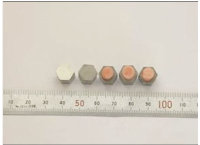
Fig. 2. Samples (Co-Cr alloy, Sandblasted specimen, Resin-bonded Specimens).
