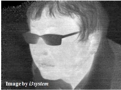
Figure 7. Thermographic still image of room-temperature (300 K) object taken by [320×256]-FPA thermographic module (77 K) of p-i-n SLIP.
