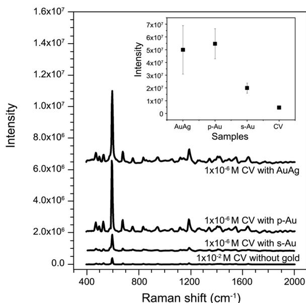
**Figure 2.** Raman spectra for the CV probe molecules with the gold nanomaterials; AuAg alloy, p-Au, and s-Au NWs. Inset is the SERS intensity measured at  $592\text{ cm}^{-1}$  with an error range for a better comparison.
