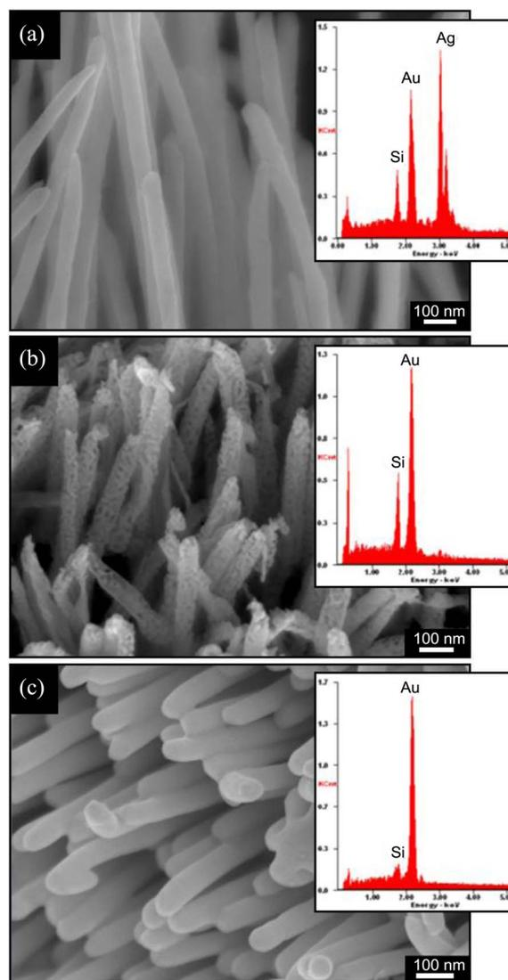
**Figure 1.** SEM images and EDX spectra (insets) of the AuAg alloy (a), p-Au (b), and s-Au (c) nanowires. The samples are dispersed on silicon wafers for the measurements.
