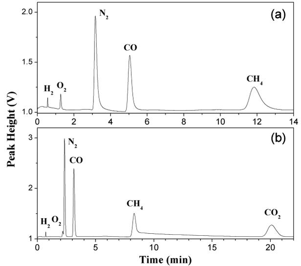
**Fig. 5.** Chromatograms for the H<sub>2</sub>/CH<sub>4</sub>/CO/CO<sub>2</sub> mixture gas measured with (a) a Molsieve 13X and (b) a Carboxen 1000 packed column.
