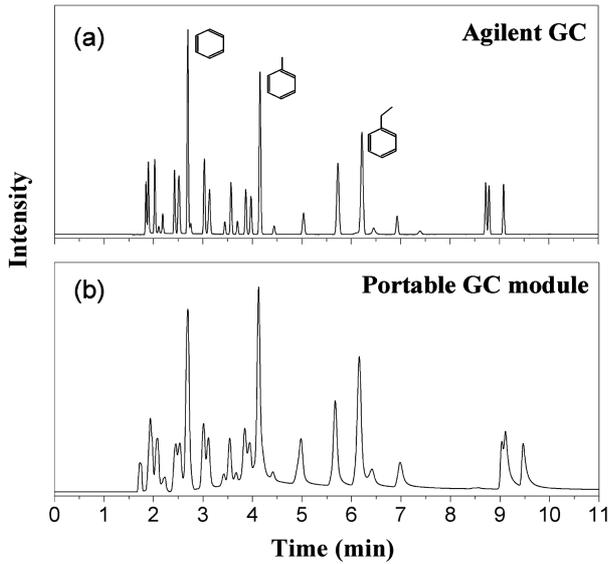
**Fig. 4.** Comparison of chromatograms showing the analysis of the 26-component mixture measured with (a) an Agilent 7890A GC and (b) the portable GC module.
