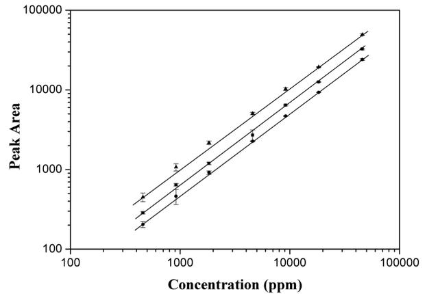
Fig. 7. Calibration curves of three different gases measured with a Carbosieve S-II packed column. ●, CH<sub>4</sub>; ■, CO; ▲, CO<sub>2</sub>.
