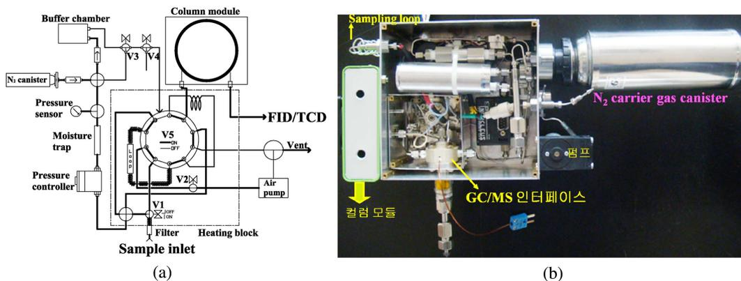
Fig. 1. (a) Schematic diagram of a portable GC module. (b) Portable GC module.
