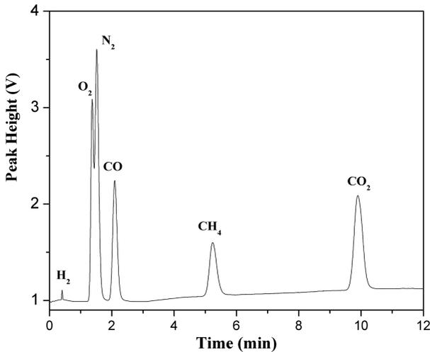
Fig. 6. Chromatogram of H<sub>2</sub>/CH<sub>4</sub>/N<sub>2</sub>/O<sub>2</sub>/CO/CO<sub>2</sub> mixture gas measured with a Carbosieve S-II packed column and a TCD.
