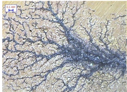
Fig. 4. A magnified carbonized surface tracking pattern photographed by an optical microscope.
