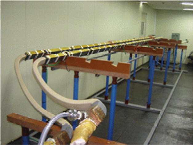
Fig. 1. Accelerated aging tests for generator stator bars #1 and #2
