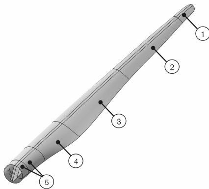
Fig. 7 Blade Regions according to Variable Lay-up Pattern & Thickness
