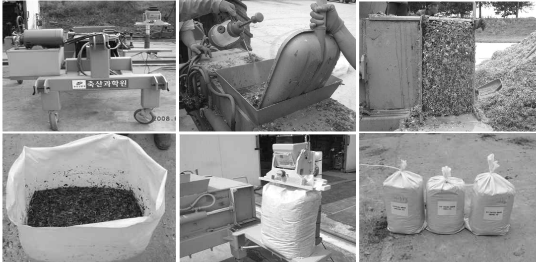
Fig. 1. Making of corn silage using square silage wrapping compressor.
