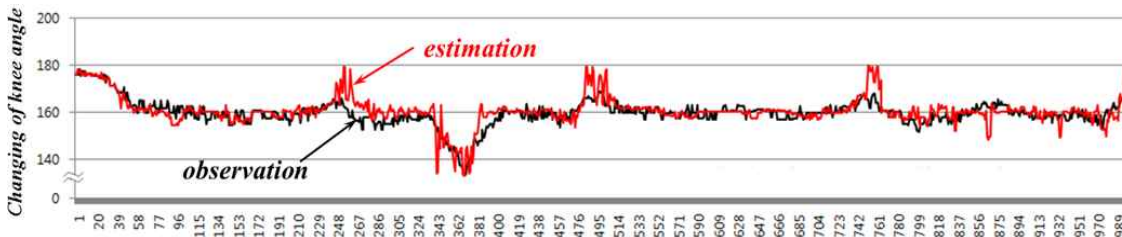
Fig. 9. The graph compares the k-NN based estimated posture result with the ground-truth by observed camera without angle consistency.
