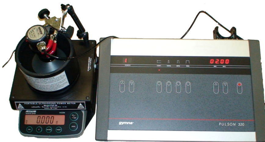
Figure 1. Illustration of the power output testing procedure.
