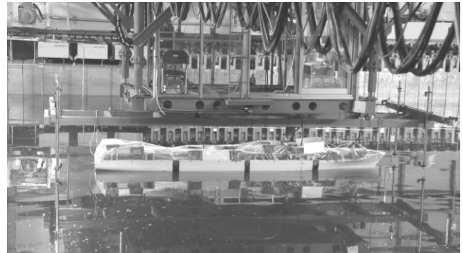
Fig. 3 Segmented model test of a container carrier at the ocean wave basin of MOERI.
