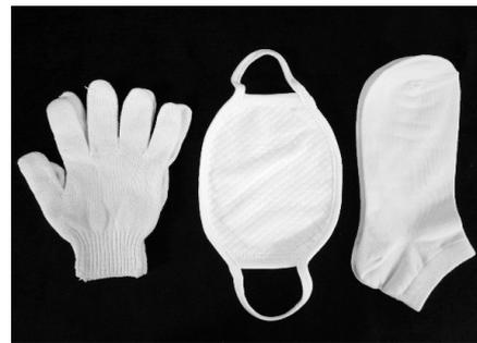
**Fig. 3.** Gloves, mask and socks for dermal exposure monitoring.
