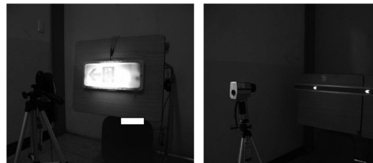
a) A testing of egress guide-light's illuminance b) A testing of egress guide-line's luminance
