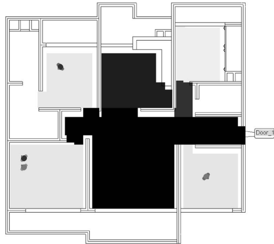
Figure 4. Spread of smoke and populations on 60 seconds after fire.
